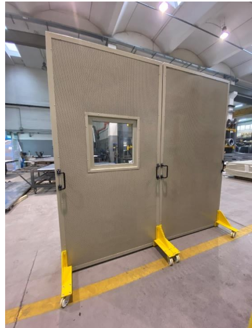
Barrier performance measured in the workplace. Barrier dimensions: 1300xH2500mm. Measurement performed at 1m distance
